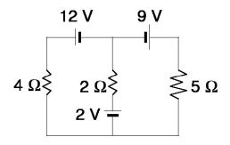
Example 4: The circuit consists of three batteries and three resistors as shown. a) Label the circuit and write down Kirchoff's loop and junction rules for the circuit. b) Find all the currents in the circuit!c) What is the total power dissipated in the circuit? d) What is the total power delivered by the three batteries in the circuit?
